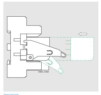
The LZS:PT17021 and LZS:PT17024 ejection brackets of the plug-in relays are not status displays!
