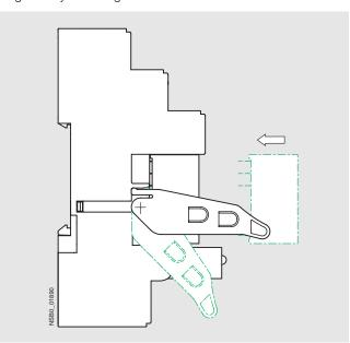
The LZS:RT17016 ejection brackets of the plug-in relays are not status displays!
